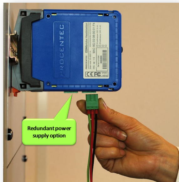
Powering the Head Station
