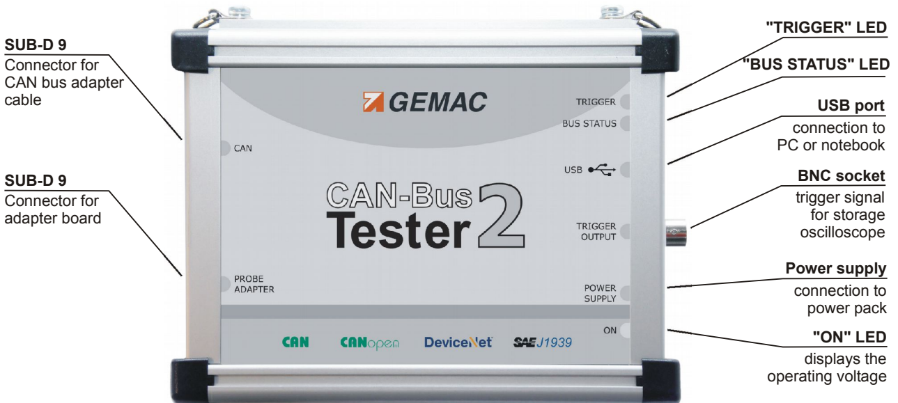
Figure 1: Connections of the CBT2
